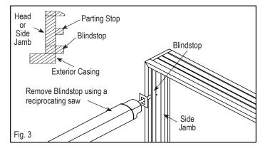
See Fig. 3. Using a reciprocating saw, remove the blindstops from the side jambs and head jamb by cutting it flush with the frame or exterior casing.
