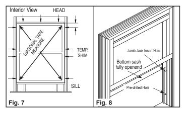
See Fig. 8. Fully open the bottom sash. There is one predrilled hole on each side jamb and one jamb jack insert on each side jamb. A second pre-drilled hole will be provided between the first pre-drilled hole and the jamb jack insert hole if the bottom sash glasss height is 30" (762mm) or greater.
