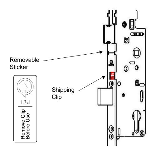
Remove shipping clip before operating multipoint gear system.
