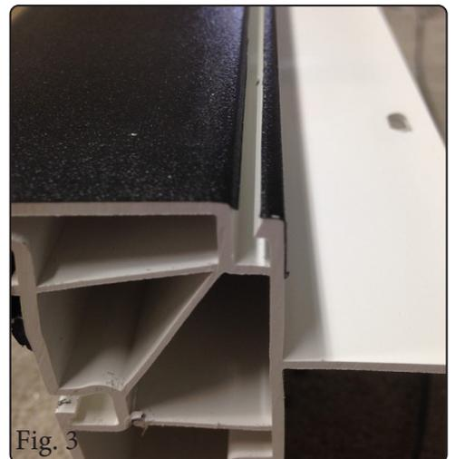
See **Fig. 2**. Score the other side of the accessory groove with the utility knife. Remove the small strip of foil from the frame.
