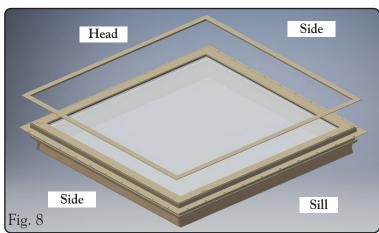
See Fig. 8. After the unit has been properly installed, apply the head j-channel to the frame by using a rubber hammer and taping it into the accessory groove. Apply the sill j-channel into the frame accessory groove the same way. Once the head and sill j-channels are installed, install the left and right j-channel pieces to the exterior starting at the head first to ensure a proper joint. Use the rubber hammer to tap into place.
